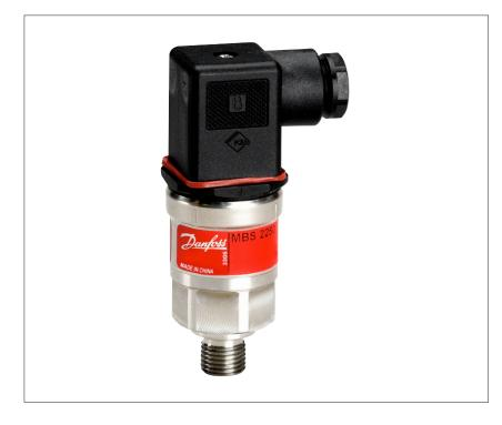
The compact heavy duty pressure transmitter type MBS 2200 and MBS 2250 are designed for use in severe industrial and hydraulic applications. MBS 2250 with integrated pulsesnubber is suitable for use in applications with severe medium influences like cavitation, liquid hammer or pressure peaks and offers a reliable pressure measurement, even under harsh environmental conditions.
