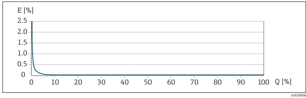
E Maximum measurement error in % o.r. (example with PremiumCal)
