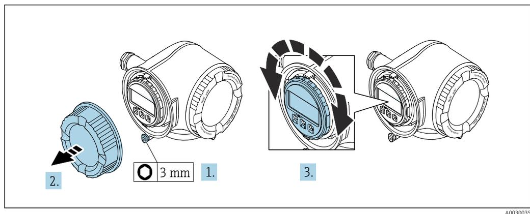
1. Depending on the device version: Loosen the securing clamp of the connection compartment cover.
