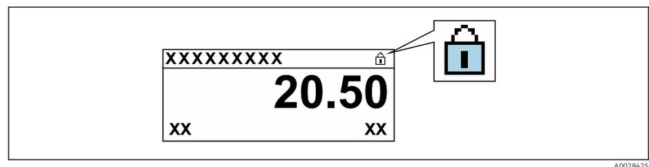
2. Setting the write protection (WP) switch on the main electronics module to the **OFF** position (factory setting) disables hardware write protection.
