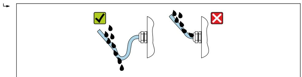
6. The cable glands supplied do not ensure housing protection when not in use. They must therefore be replaced by dummy plugs corresponding to the housing protection.
